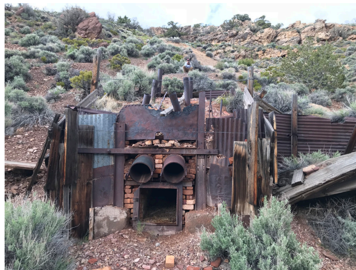
Mercury retort in Mineral County Nevada
