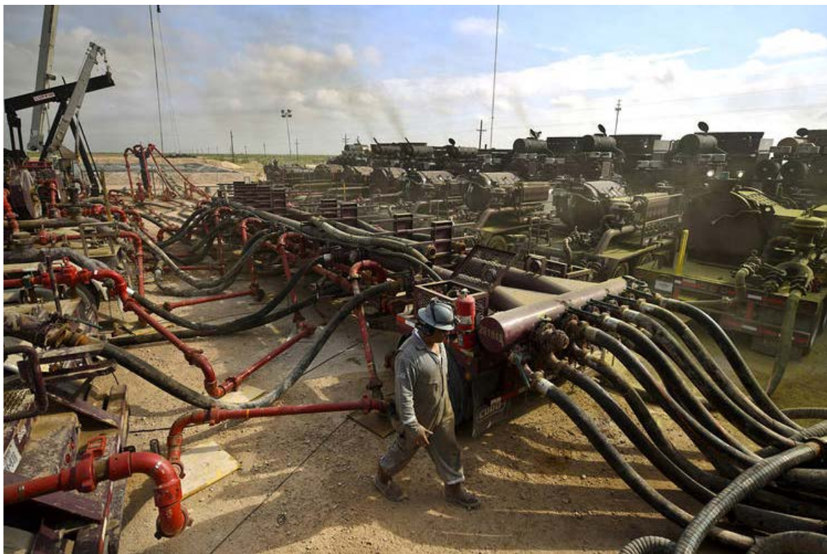
Modern fracking operations are significantly larger and more involved. Here, line boss David Cantu checks the performance of pumping units at a Cudd Energy fracking operation on a Fasken Oil and Ranch well in Midland, Texas, in May. PHOTO: JAMES DURBIN FOR THE WALL STREET JOURNAL
