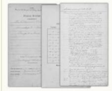
Field notes are the narrative record of the cadastral survey. They are written in tabular format and contain the detailed descriptions of entire survey process including the instrumentation and procedures utilized, calling all physical evidence evaluated in the survey proces
