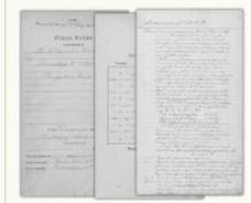
Field notes are the narrative record of the cadastral survey. They are written in tabular format and contain the detailed descriptions of entire survey process including the instrumentation and procedures utilized, calling all physical evidence evaluated in the survey proce-
