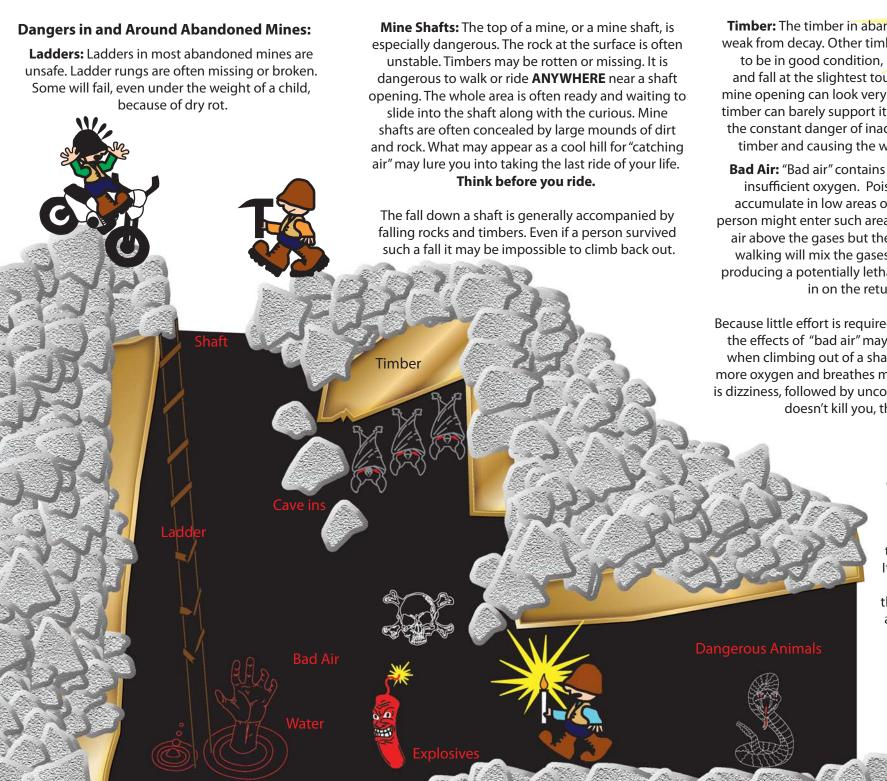
**Timber:** The timber in abandoned mines can be weak from decay. Other timber, which may appear to be in good condition, may become loose and fall at the slightest touch. A well-timbered mine opening can look very solid when in fact the timber can barely support its own weight. There is the constant danger of inadvertently touching a timber and causing the workings to collapse.
