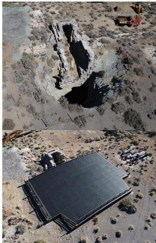
Photo 7 – Before and after photos of the Forman Shaft permanent closure.
