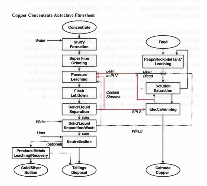
The solid residue from the solid-liquid separation step contains gold and silver, if present. The gold and silver can be recovered by neutralization with lime followed by cyanide leaching in tanks and adsorption onto activated carbon. Arsenic, bismuth and other penalty elements will be
