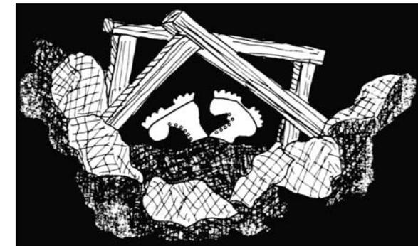
slightest touch. A well-timbered mine opening can look very solid when in fact the timber can barely support its own weight. There is the constant danger of inadvertently touching a timber and causing the tunnel to collapse.
